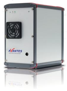
Avantes offers a wide range of NIR spectrometers. The 2.x-series extended InGaAs instruments feature 256 or 512 pixel detectors and are available in configurations enabling measurements up to 2000, 2200 and 2500 nm. Resolution can be as high as 4 nm (on the 512 pixel version) or 10 nm (256 pixel). Integration times can go as low as 10 microseconds. Three different gratings are possible.
