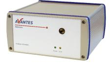
For high sensitivity applications where high resolution is not of paramount concern, the AvaSpec-HS2048XL is an exceptional instrument. Featuring Avantes' HS optical bench which has a full 0.22 numerical aperture for superior throughput, the AvaSpec-HS2048XL has a back-thinned CCD detector with 2048 pixels measuring 14X500 microns.
